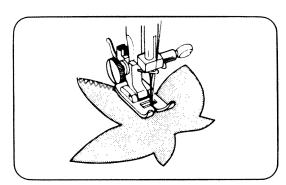
To change direction at corners, or to sew very small circles, stop machine, positioning needle just away from edge of cut-out, lift presser foot and turn material. Lower presser foot and continue sewing.
